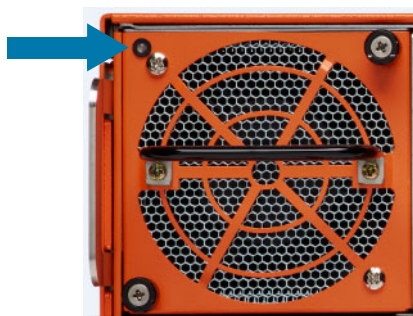
Figure 4-6: Individual Fan LED Location on GigaVUE-HC3 Rear
