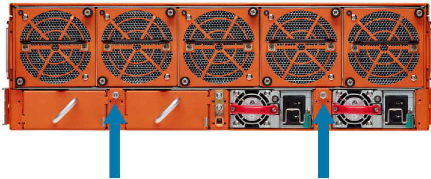
Figure 4-10: Fan Tray Screw Location on GigaVUE-HC3 Rear
